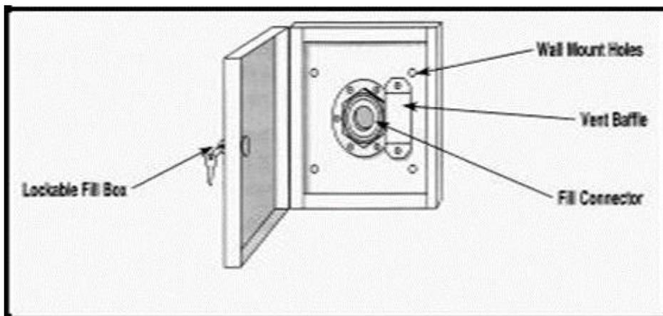
6. Pass the fill line through the wall, and mark for cutting to length. Pull the fill box back off the wall. Cut fill line to length, then cut vent line to same length, and secure with screw to bracket in back of fill box.
