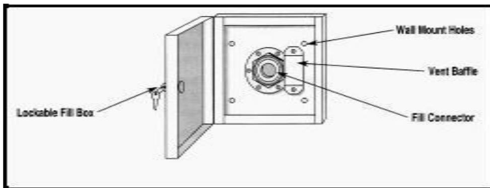
6. Pass the fill line through the wall, and mark for cutting to length. Pull the fill box back off the wall. Cut fill line to length, then cut vent line to same length, and secure with screw to bracket in back of fill box.
