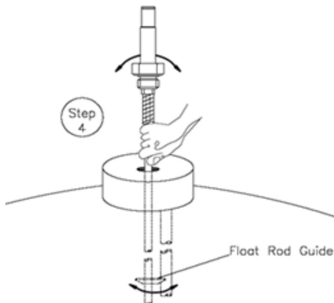
5. When the rod is engaged in the guide ring, the rod will be restricted to lower end movement of about  $\frac{1}{2}$  in. (12.7 mm); if you can feel greater movement, withdraw the rod to the point where its top is 8 in. (203 mm) above the gauge opening and try again.
