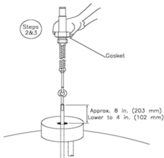
4. To confirm that the rod is correctly positioned in the container, stop where you can still grasp the top of the rod and try to swing the lower end from side to side.
